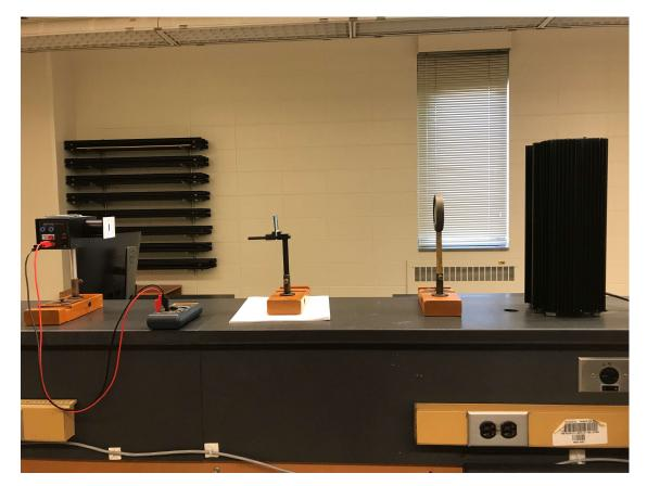
1.4. Make sure that a single vertical slit is covering the front opening of the mercury lamp.
