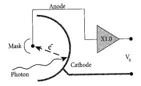
Some photoelectrons travel toward the stopping electrode (anode) and, upon reaching it, constitute a current, which flows through the circuit. As we increase the voltage V, some of the less energetic photoelectrons will be repelled from the anode and the current will decrease. At some voltage  $V = V_S$  (the stopping voltage), the most energetic photoelectrons will be stopped just in front of the anode and current will cease to flow. For this condition:
