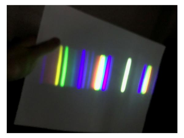
1.10. The diffraction grating separates these lines, so we will use only one color (i.e., one wavelength) at a time. Please recall your observations from the last part the "Diffraction Grating" experiment. To make the separation of lines even better, use yellow and green filters for yellow and green lines, respectively. These filters have magnets built in, so
